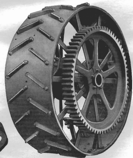
Standard Drive Wheel Showing Master Gear Attached
